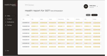
The device Health Report screen allows the user to track the health of a specific device and plan any future service actions.
